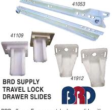
BRD offers a European style drawer slide with the RV front Drop Lock feature. Drawer slides allow the drawer to lift up and glide out on two solid stud acetal rollers. Single captive design allows the slide to adjust to the constant movement of an RV. These slides allow easy installation with a front tab mounting feature.
